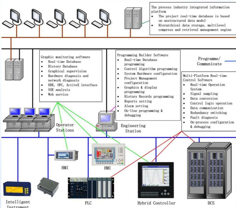
UWinRDB is used to define Tags information of each station, including the station's component instrumentations and attributions, each Tag's attributions such as data acquisition & conversion, alarm, history recording, security zone, etc; Realizes globally consistent & unified interface.
